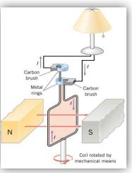
You have made a simple generator to power a TV. The armature is attached the rear axle of a stationary bike. For every time you peddle, the rear axel turns 10 times. Your TV needs a  $V_{rms}$  of 110V to operate. If the B-field is 0.2 T, each loop is a circle with r = 3 cm, and you can comfortably peddle 3 times a second; how many loops must you have in your generator so that you can watch TV while you exercise?
